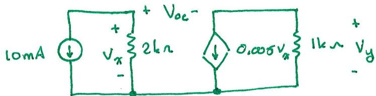
$$V_x = -(2k\Omega)(10\text{mA}) = -20\text{V}$$
