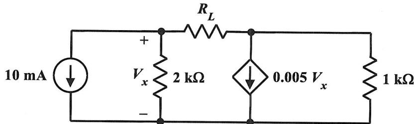
What value of  $R_L$  will absorb maximum power from the remainder of the circuit?
